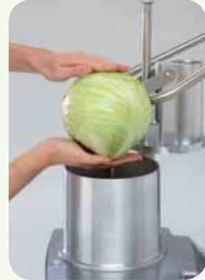
**Power lever** to take the strain and increase throughput.
