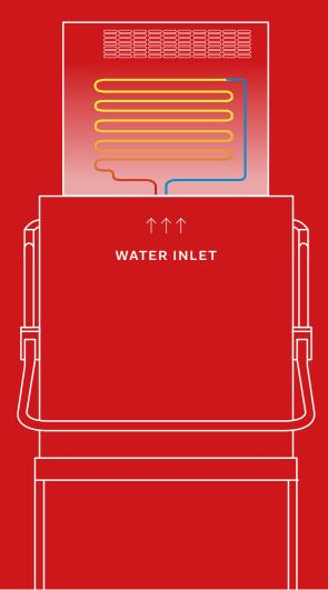
This system helps to minimize the steam released to **create a more comfortable work environment** while using the warmth of the unit to further heat incoming water and reduce energy costs. That reduction of steam in the washing chamber also contributes to speedier drying of glasses and dishes. -35% Energy consumption
