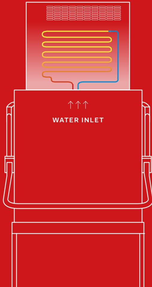
This system helps to minimize the steam released to **create a more comfortable work environment** while using the warmth of the unit to further heat incoming water and reduce energy costs. That reduction of steam in the washing chamber also contributes to speedier drying of glasses and dishes.
