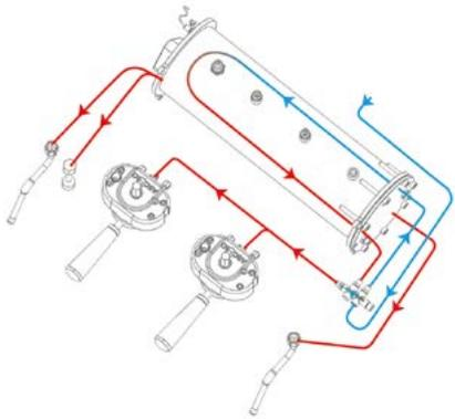
The multi-group technology is based on coffee groups and a steam boiler that work completely independently. Each group and boiler have their own autonomous heating system, safety device and precise electronic temperature control.
