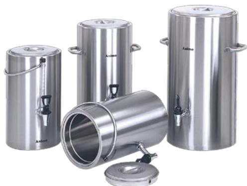
**CE-series:** equipped with a heating element with klixon thermostat that does not touch the bottom. This gives a hot air au bain-marie effect that maintains the proper temperature of the beverage (about 85 °C) and it can be kept for a longer time. Options: 4, 6, 8, 10, 12, 16, 20 or 25 litres. 4 - 8 litre containers have a carrying bracket, the others have grips.
