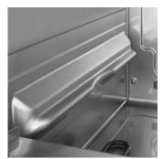
Fitting the grille in the wash chamber is a quick and simple operation: just rest it on the supports provided.
