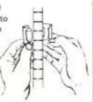
Tapered collars in each corner of shelf slide over plastic clips. As shelf load increases, wedge lock action increases in strength.
