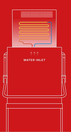
This system helps to minimize the steam released to **create** a more comfortable work environment while using the warmth of the unit to further heat incoming water and reduce energy costs. That reduction of steam in the washing chamber also contributes to speedier drying of glasses and dishes.
