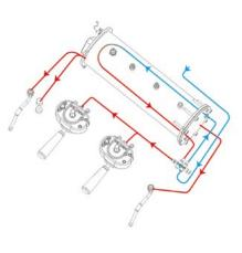
The multi-group technology is based on coffee groups and a steam boiler that work completely independently. Each group and boiler have their own autonomous heating system, safety device and precise electronic temperature control.
