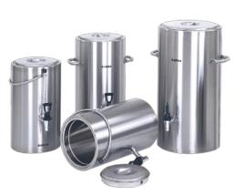
**CE-series:** equipped with a heating element with klixon thermostat that does not touch the bottom. This gives a hot air au bain-marie effect that maintains the proper temperature of the beverage (about 85 °C) and it can be kept for a longer time. Options: 4, 6, 8, 10, 12, 16, 20 or 25 litres. 4 - 8 litre containers have a carrying bracket, the others have grips.
